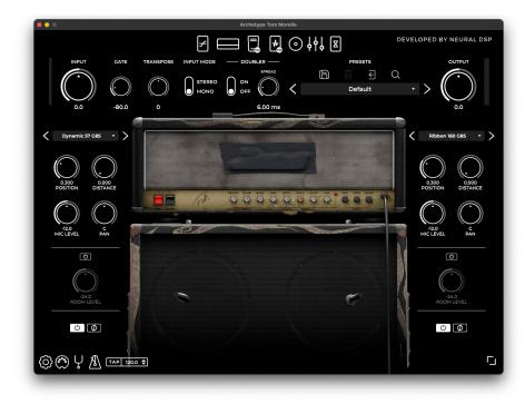
The cabinet section features 10 different microphones with a range of different positions.
